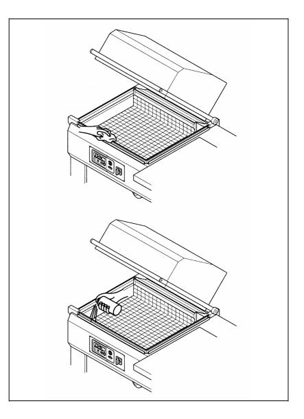
Lubricate the welding blade periodically with the supplied non-adhesive spray.
