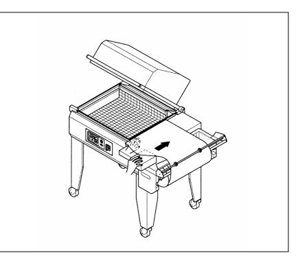
By pushing the cover handle with a pressure of 10-15 Kg. the cover rests on the sealing blade; by pinching the film, it is automatically sealed on the open sides (right and front). In case you have selected the function "SEALING +
