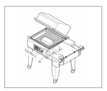
Place film as shown in the picture to carry out the first seal.
