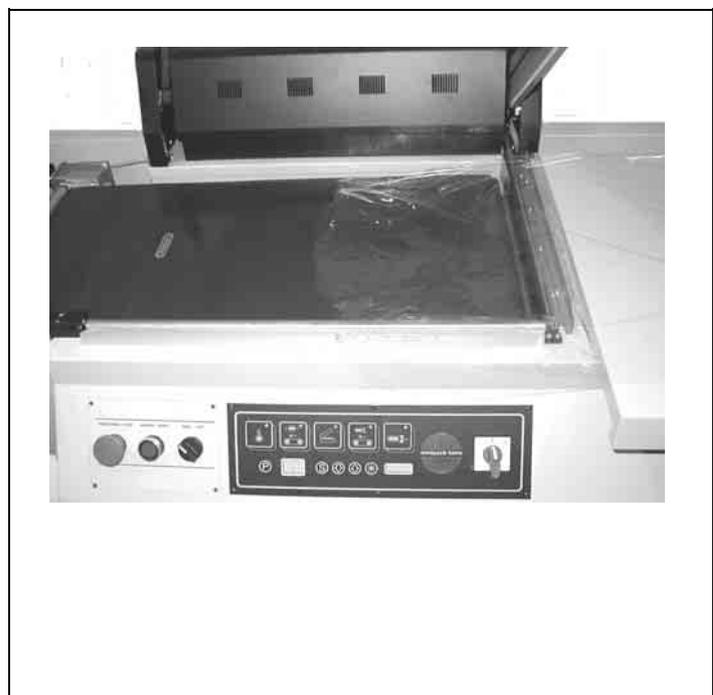
Rotate the selector (Q) to MANUAL-position and press the start button (P). The machine will automatically start operating, and the first welding will be
