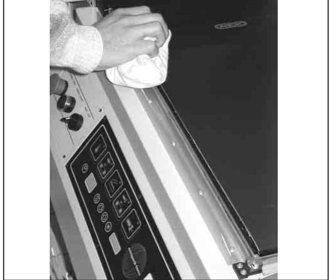
*Lubricate the welding blade periodically with the supplied non-adhesive spray*
