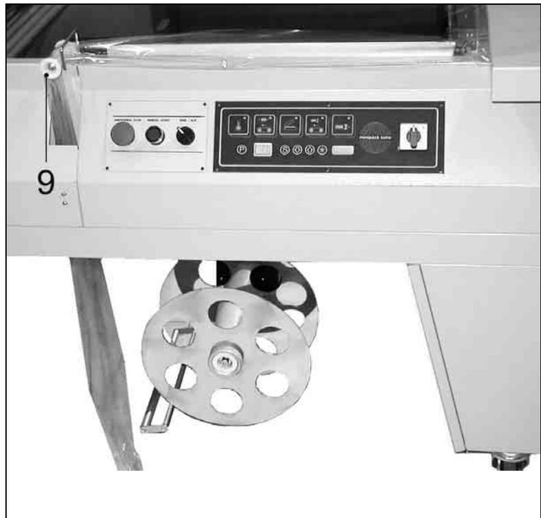
Guide this film strip around the transmission roll (9) and the driving roll (10) and couple it with the coiler (11). The machine is now ready to start the packaging.
